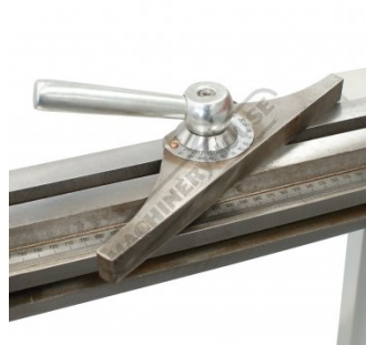
Adjustable and sliding mitre guide
