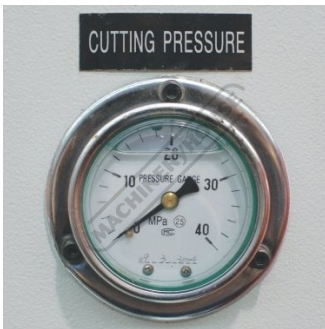
Cutting Pressure Gauge
