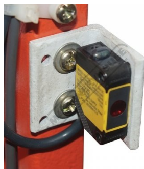
Safety Omron E3ZS Rear Light Sensor Guarding
