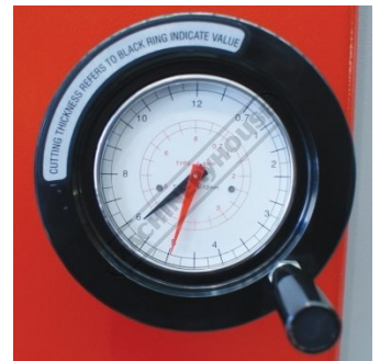
Variable Blade Gap Adjustment Dial
