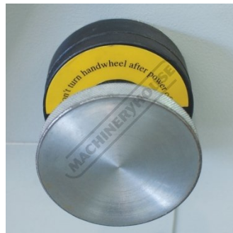
Fine Adjustment Dial for Backgauge
