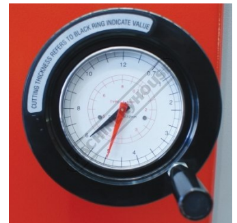
Variable Blade Gap Adjustment Dial
