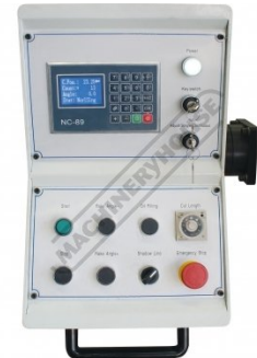
Controller with NC 89
