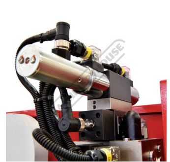
Safety Monitoring Valve
