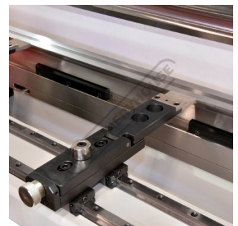
Micro Adjustment Backstop
