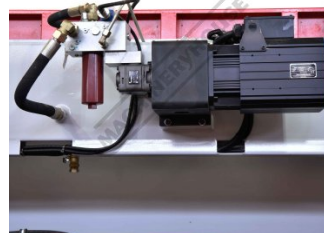
Eco Friendly Servo Driven Hydraulics
