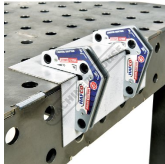
Mult Angle Magnet Shown Setup in 90 Degrees
