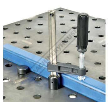
Clamp Shown Clamping Square Tube
