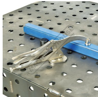
Shown Clamping Square Tube
