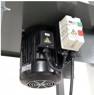
17" Impeller Driven By 5hp 415V Motor
