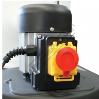
Safety Stop Switch
