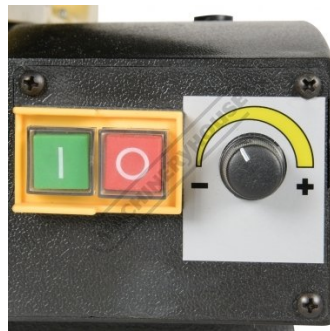
Switch And Variable Blade Speed Dial
