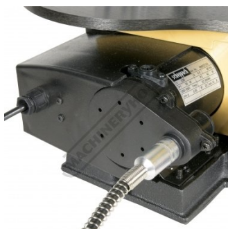
Drive Connector For Flexible Shaft Attachment
