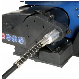
Drive Connector For Flexible Shaft Attachment
