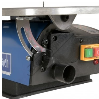
Tilt Table Adjustment & Dust Port
