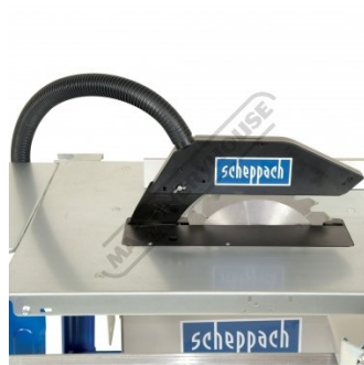
315mm Saw Blade With Blade Guard
