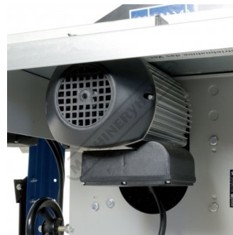
3hp 240V Induction Motor With Brake
