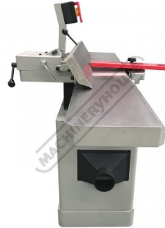
Side View with Fence at 45 Degrees
