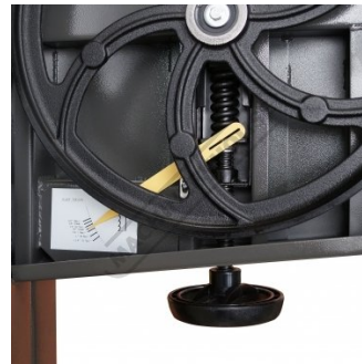
Blade Tension Hand Wheel And Guide
