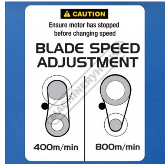
Belt Speed Diagram
